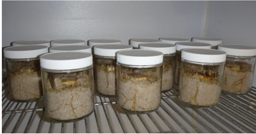
Figure 3.2 Termite jars exposed to treatments in the laboratory incubator at 25°C.
